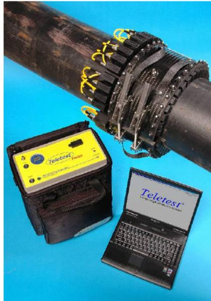
Figure 1: Multi-Mode' Teletest® Equipment
